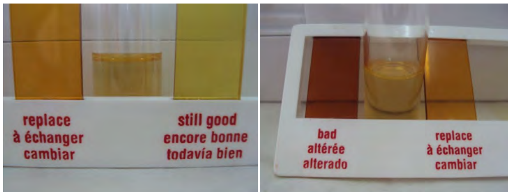
Photo 3. FRI-TEST color evolution with the cycles. The oil in left is still fit for use. In the right, the oil with 47 cycles where change is recommended but is not yet altered.
