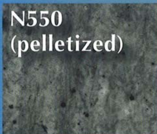
Dispersion in Low Viscosity PDMS (10 sec. Mixing)
